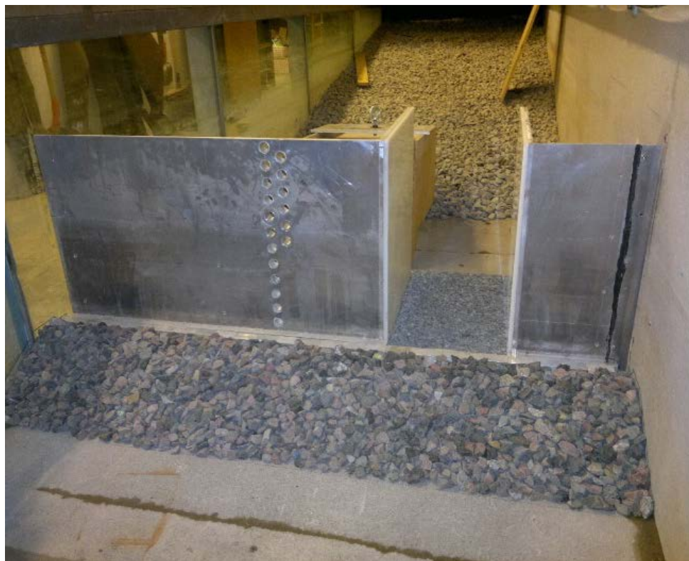
Figure 5 – The fixed caissons and the rubble mound used as foundation.
