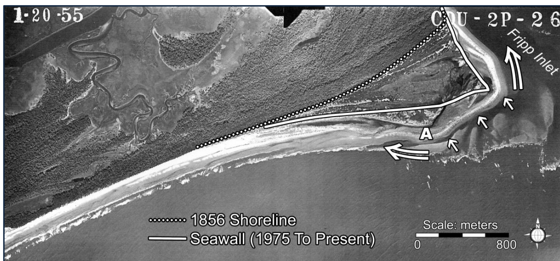
Figure 2. Vertical aerial photo of Fripp Island (January 1955 by US Department of Agriculture) showing approximate 1856 shoreline and present seawall. The island accreted via episodic shoal bypassing at Fripp Inlet (arrows) through the 1950s, then went into an erosion cycle in the 1970s after the first development.
