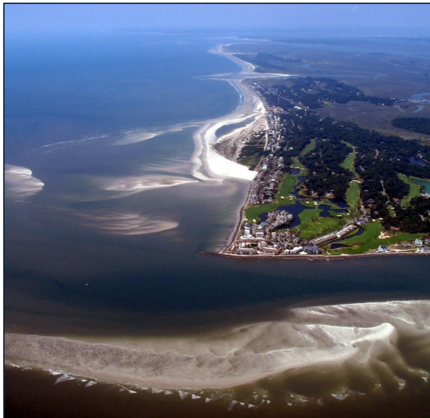
Figure 13. Oblique aerial photo at low tide on 31 May 2008 showing the accumulation of sand from recent bypassing events against the seawall along the center of Fripp Island. [Photo by TW Kana]
