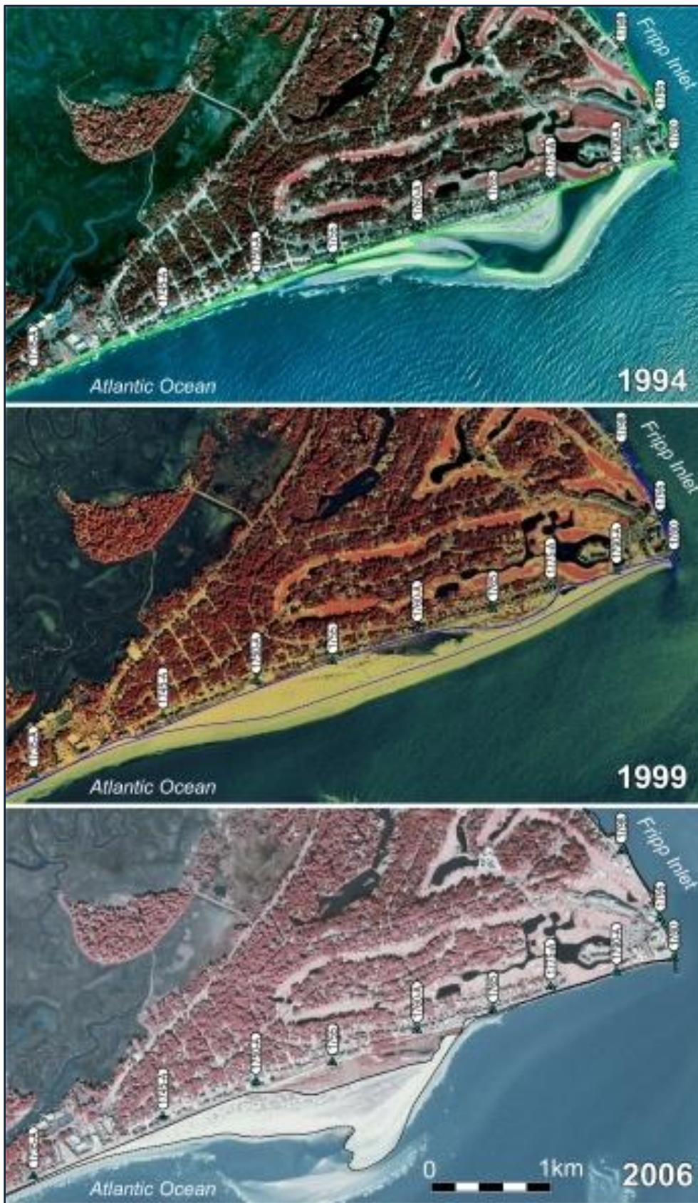
Figure 12. Sequence of vertical aerial images of Fripp Island showing the impact of episodic bypassing events at Fripp Inlet and the natural restoration of beach fronting the seawall. [Photo Source: SCDNR]
