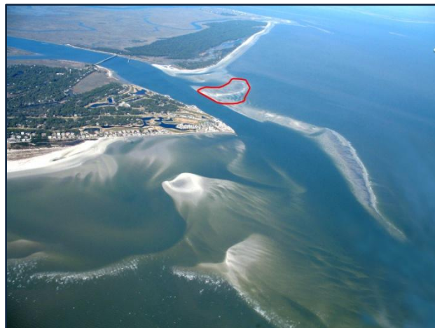
Figure 3. Fripp Inlet at low tide (February 2007) looking north, showing extension of north shoal of the ebb-tidal delta. Bypassing bar migration toward Fripp Island in foreground. Highlighted area was used as a borrow area for several nourishment projects along Hunting Island (top of photo).
