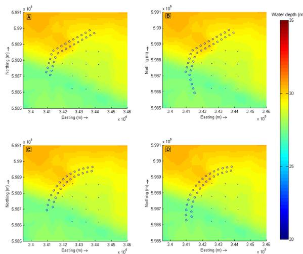
Figure 3. Co-located farm layouts. Configurations A to D and FINO1 research platform included. Values of the water depth (m).
