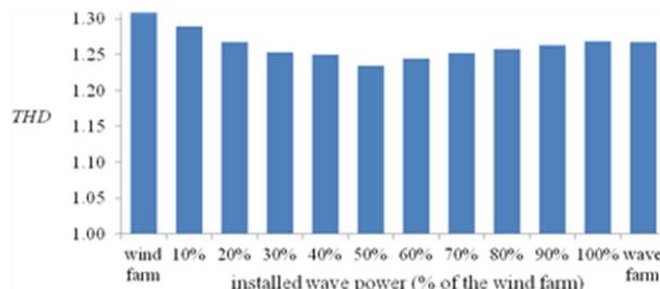
**Figure 4. Variability of the annual power output in terms of the THD indicator during the study period for the combined farms at Alpha Ventus and Horns Rev.**
