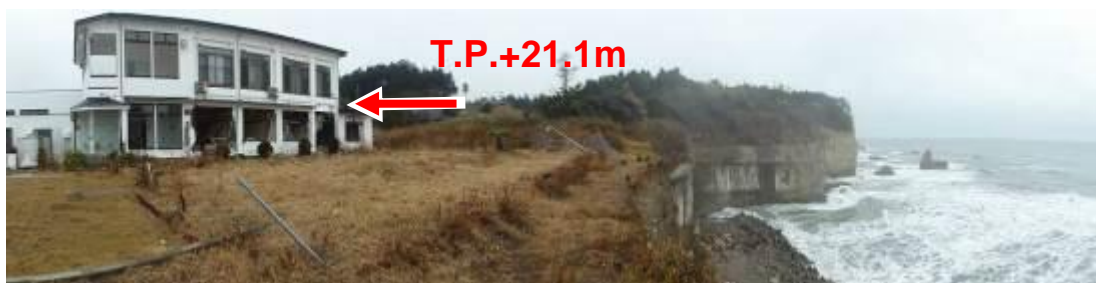
Figure 13. Highest watermark in Fukushima observed on the top of a coastal cliff in Tomioka, located between the Fukushima Dai-ichi NPP and the Fukushima Dai-ni NPP (Sato et al., 2013).
