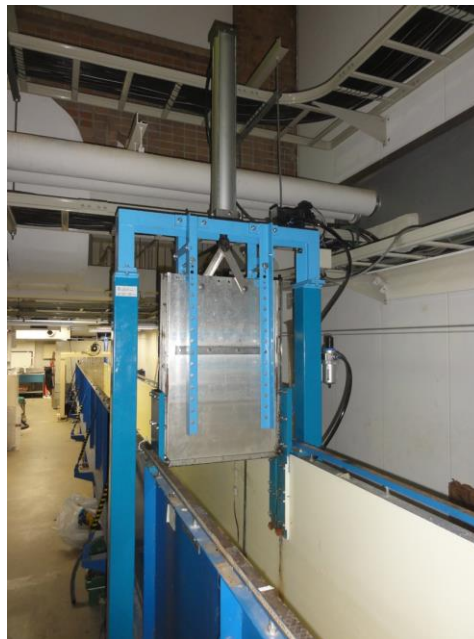
Figure 2. Hydraulically-driven dam-break gate (The speed of the gate can be changed by the oil pressure from 1 (slowest) to 6 (fastest)).
