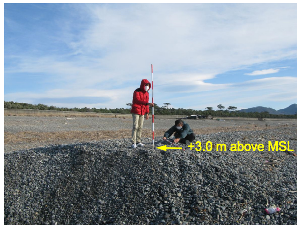
Figure 6. Berm height of 3 m above MSL immediately east of the floodway.
