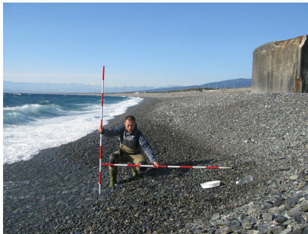
Figure 9. Foreshore slope of 1/4 at a location where filtration water discharges out to sea.
