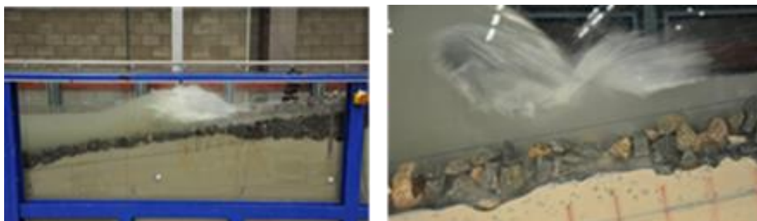
Figure 1. Open transport filters with rock on top of sand (from Van Gent and Wolters, 2015).
