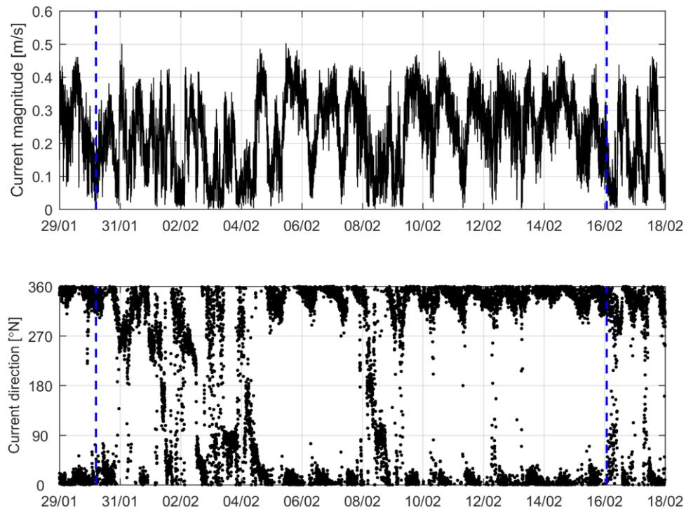
Figure 4: Part of the measured current time series (currents at  $z=0.4h$ ) during Deployment 2. Vertical dashed blue lines indicate the events that have been used for validation of the SWASH model.
