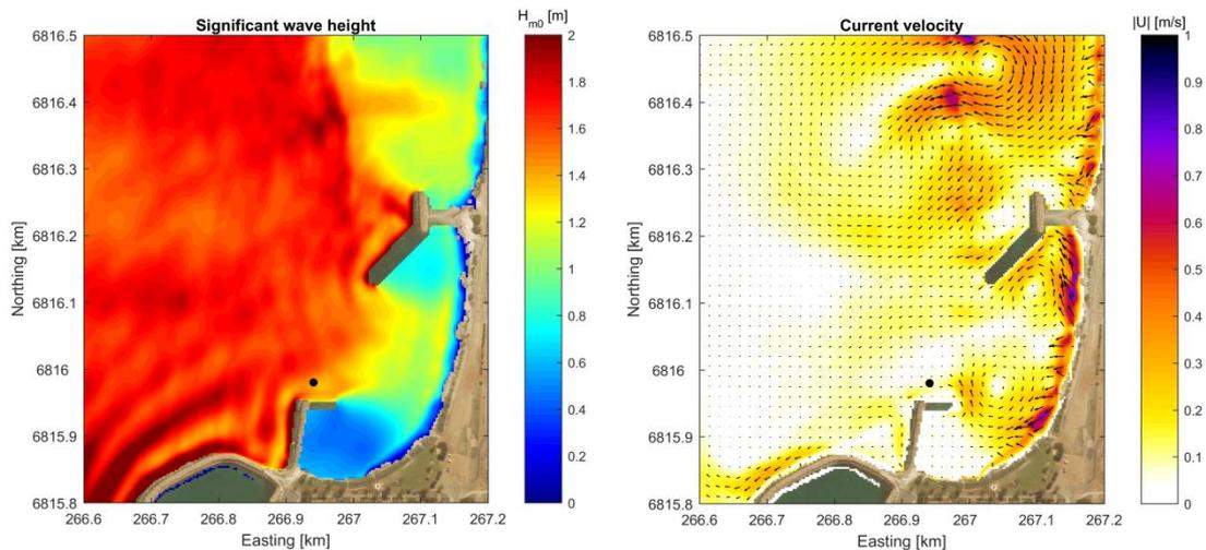
**Figure 13: Spatial distribution of the significant wave height (left) and current magnitude and direction (right) for the proposed option consisting of a 100 m breakwater extension, a connection to the shore and a 40 m spur attached to Batavia groyne. Offshore condition:  $H_{m0} = 1.5$  m,  $T_p = 12$  s and  $\theta_p = 270^\circ$ N.**
