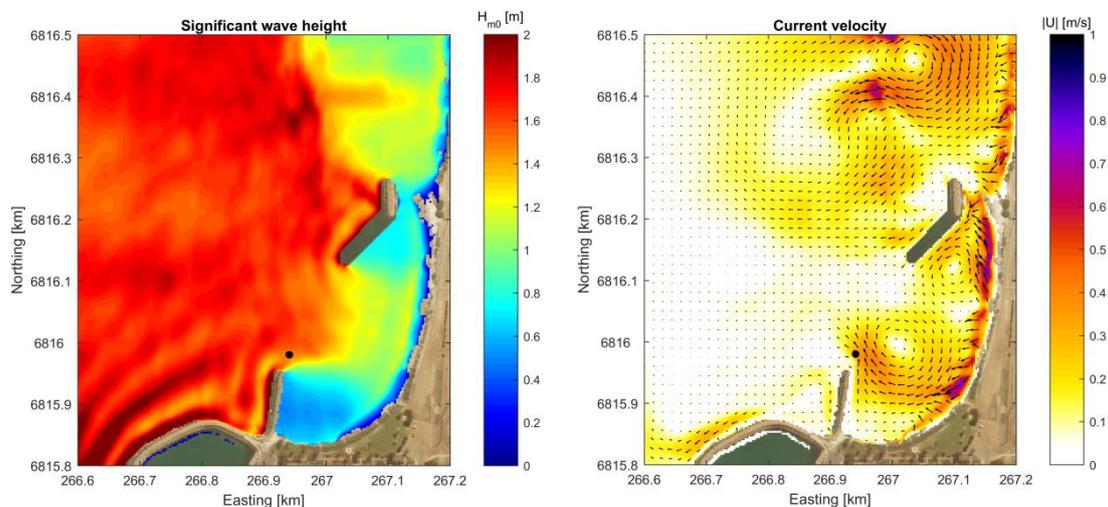
**Figure 12: Spatial distribution of the significant wave height (left) and current magnitude and direction (right) for the option with a 100 m breakwater extension. Offshore condition:  $H_{m0} = 1.5$  m,  $T_p = 12$  s and  $\theta_p = 270^\circ$ N.**
