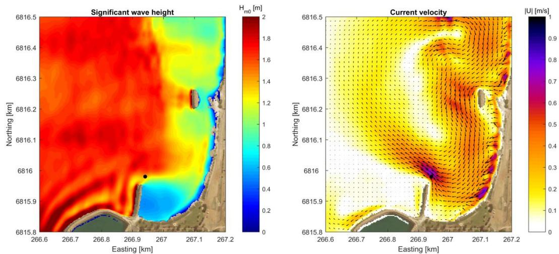
**Figure 10: Spatial distribution of the significant wave height (left) and current magnitude and direction (right) for the present situation. Offshore condition:  $H_{m0} = 1.5$  m,  $T_p = 12$  s and  $\theta_p = 270^\circ$ N.**
