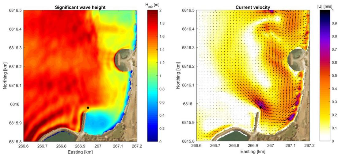
**Figure 11: Spatial distribution of the significant wave height (left) and current magnitude and direction (right) for the artificial headland option. Offshore condition:  $H_{m0} = 1.5$  m,  $T_p = 12$  s and  $\theta_p = 270^\circ$ N.**
