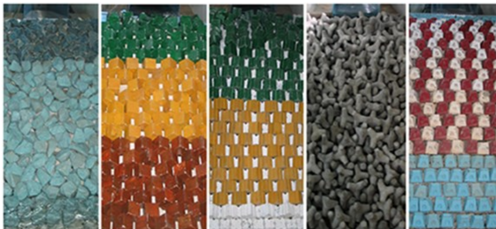
Figure 5. Model of Rock, Cube, Antifer, Tetrapod and 2B Block
