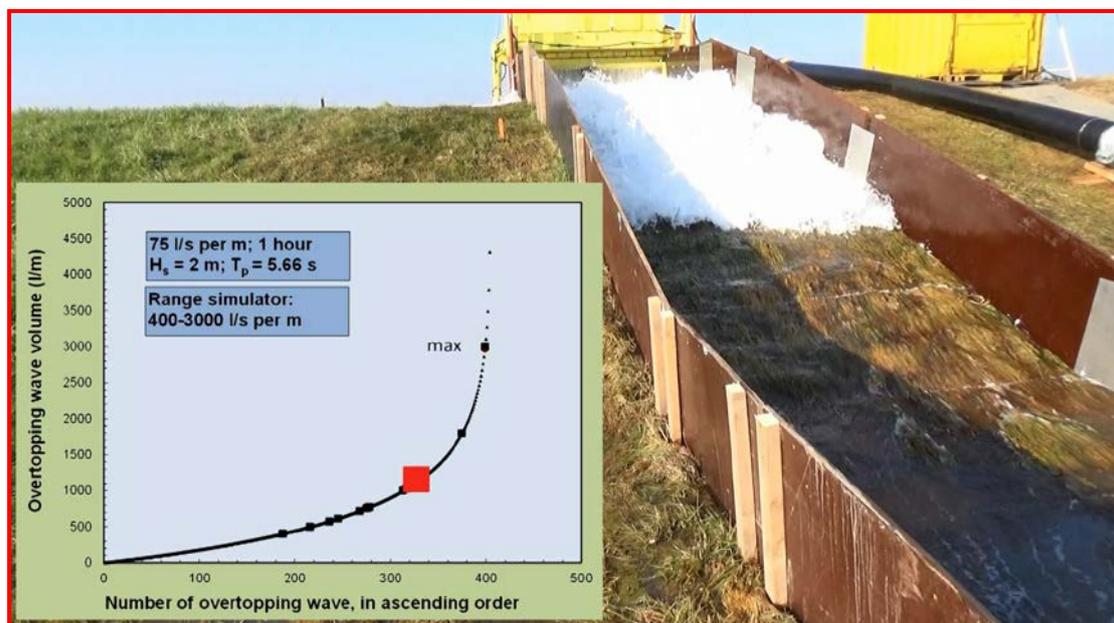
Figure 2. Snapshot of a three-minute video showing the overtopping wave volume from the wave overtopping simulator as well the size in the graph (red square)
