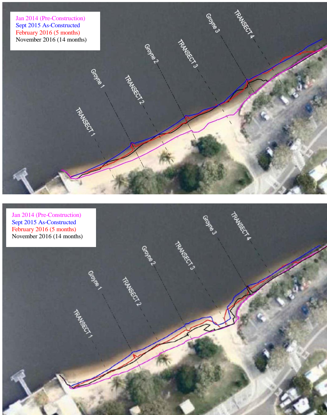
Figure 10. Monitoring Survey showing Transect Location and Planform Shape of the Beach at Mid Tide (top) and High Tide (bottom)
