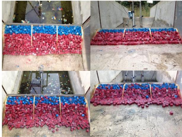
Figure 20. Pre-storm (upper) and Post-storm (lower) photos for EB. Storm condition B.
