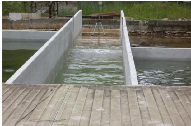
**Figure 6. Tests for wave measurements at the toe of the wall.**
