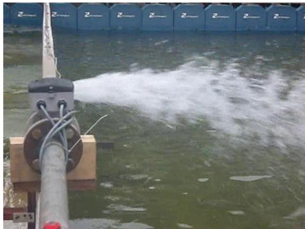
**Figure 7. View of the electromagnetic flow meter.**
