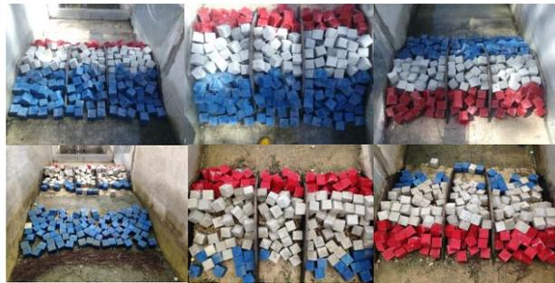
Figure 19. Pre-storm (upper) and post-storm (lower) photos for LCB. Storm condition B.
