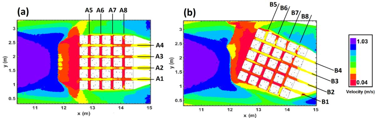
Fig. 3. The velocity distribution for the (a) aligned city buildings and the (b) skewed city buildings relative to the incoming flow at  $T=5.0$  s
