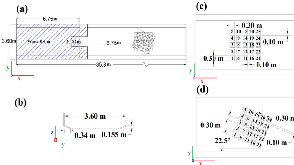
Fig. 1. The model setup: (a) the schematic view for the model setup, (b) the channel cross section, (c) buildings aligned at a zero (Case 1) and (d) buildings aligned at  $22.5^\circ$  angle relative to the approach flow direction (Case 2)
