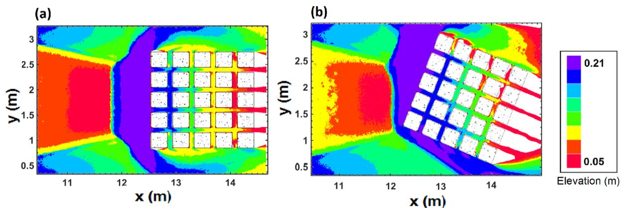
Fig. 2: The water elevation distribution at  $T=5$  s and for buildings aligned at a (a) zero and (b)  $22.5^\circ$  angle relative to the approach flow direction.
