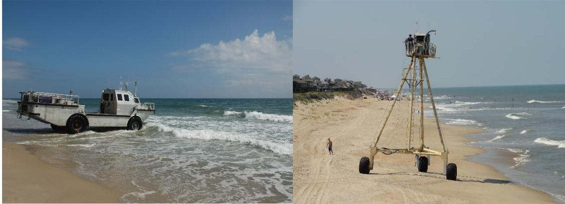
Figure 1. FRF Bathymetric Survey Vehicles LARC (left panel) and CRAB (right panel).
