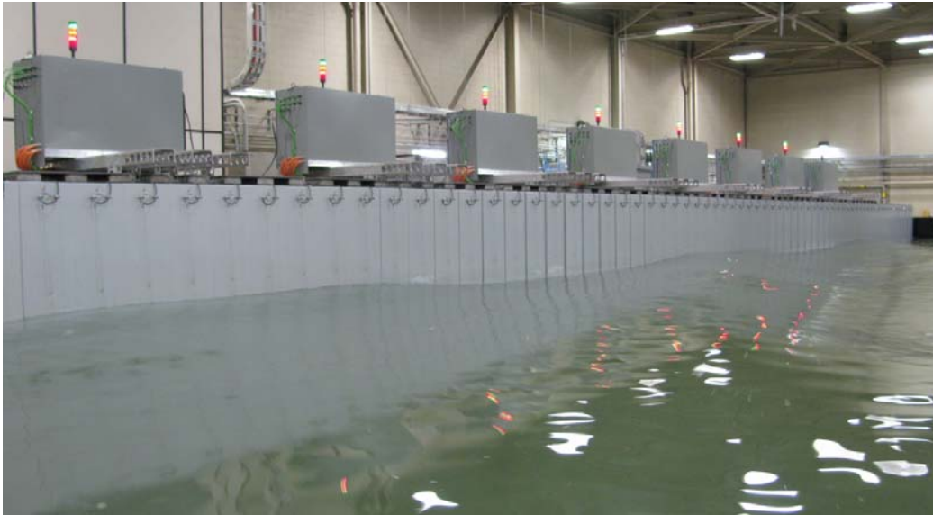
Figure 1. New 72-segment portable directional wave generator.
