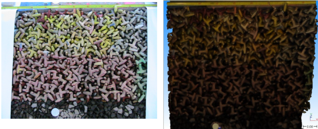
Figure 2: Camera image of dolos slope (Left) , 3D laser scanner image of dolos slope (Right).
