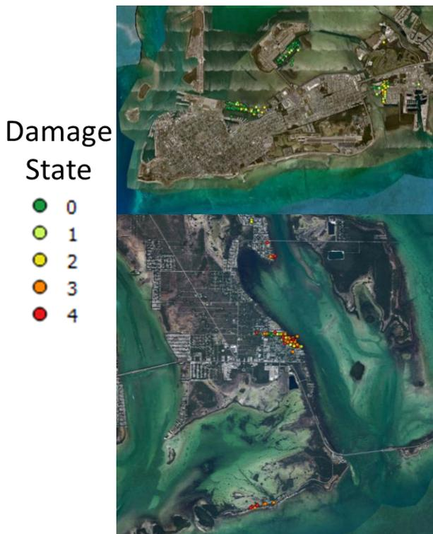
Figure 1: Top- damage to residential structures in (top) Key West and (bottom) Big Pine Key after Hurricane Irma.
