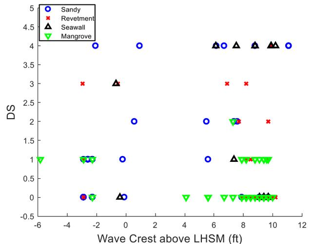
Figure 2: Structural damage state plotted against the elevation of wave crest above the structure's lowest horizontal structural member, classified by shoreline type: sandy beach (blue circles), revetment (red exes), seawall (black upward triangles), and mangrove (green downward triangles).
