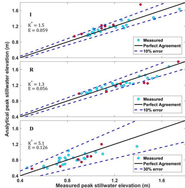
Figure 2 Measured and analytical peak still-water elevations in bay at tide gauges I ( $K^* = 1.5$ ), R ( $K^* = 1.3$ ), and D ( $K^* = 5.1$ ) with 10% or 30% error range and RMS relative error E.
