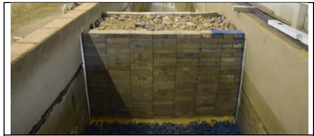
Figure 2 Example blockwork breakwater before testing
