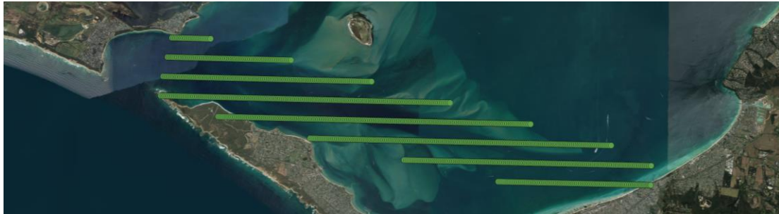
Figure 5. Output locations for Delft3D generated hydrodynamic data for tidal sand wave prediction in South Channel. Every data point provides a value for the water depth and M2 tidal velocity.
