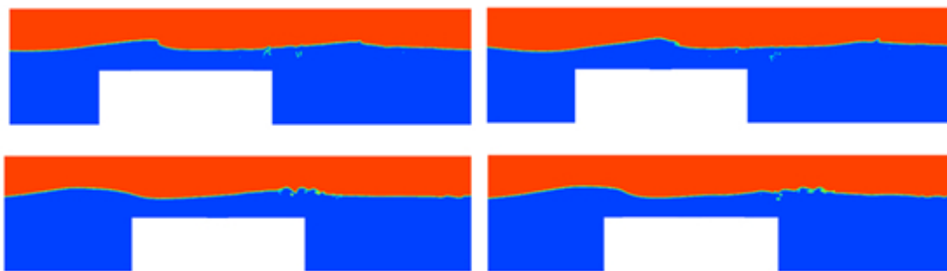
Figure 8: The breaking of waves passing over the roof of the submerged breakwater.
