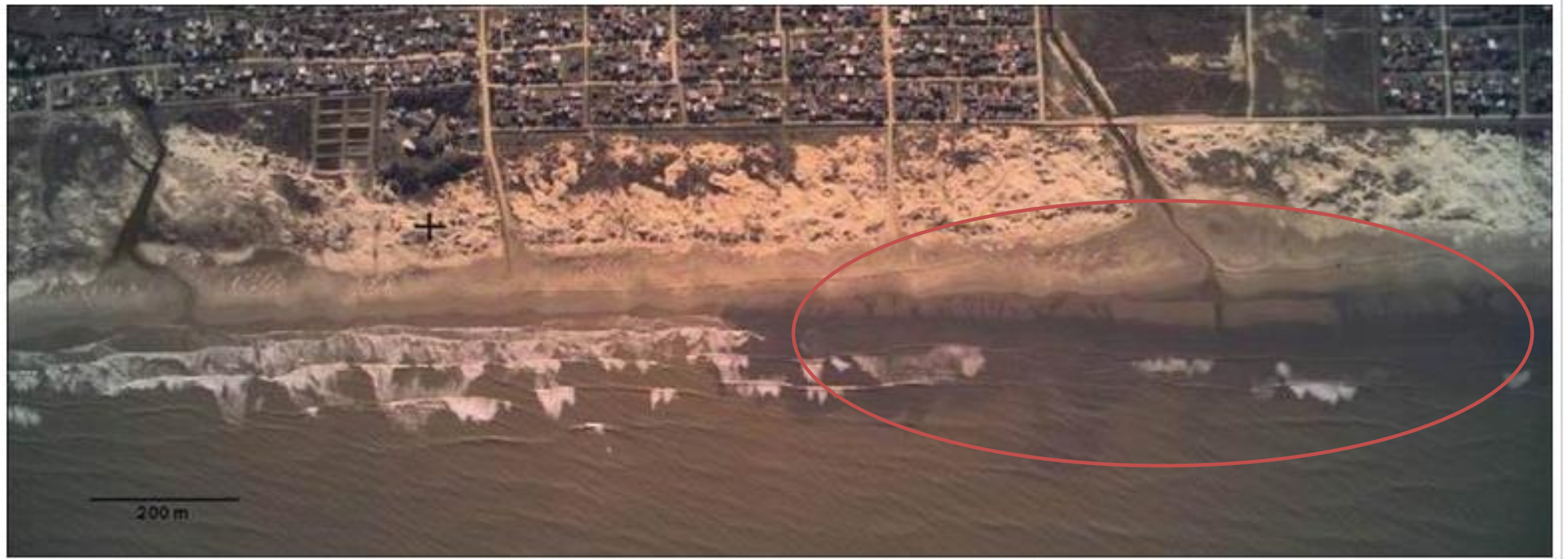
[14] “1998 Airborne Data Acquisition and Registration (ADAR) image showing differential wave breaking due to shallow water mud deposits at the landward location of the field experiment.”, (from K.T.Hollandetal./Continental Shelf Research 29 (2009) 503–514
