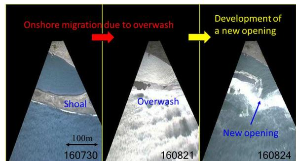
Figure 5 - Onshore migration of a shoal due to overwash and development of a new opening after high waves. Each of the three images is an ortho-image.
