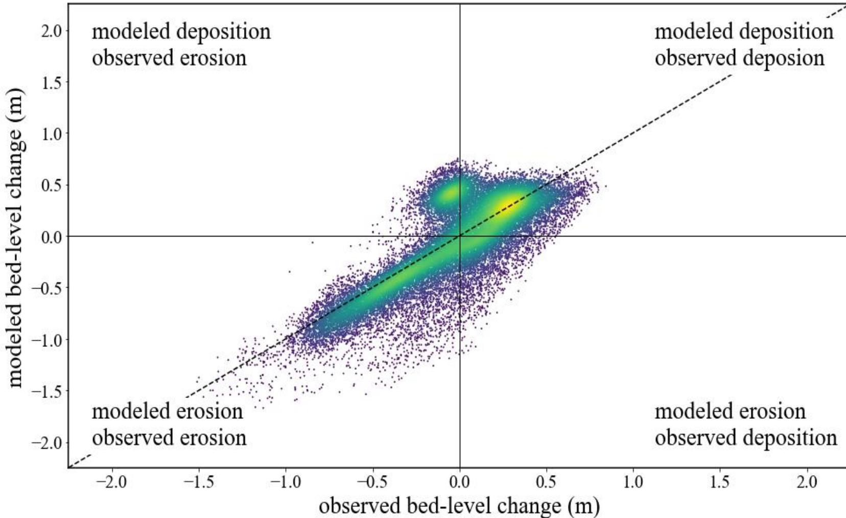
$$Skill = 1 - \frac{\sum_{i=1}^N (\Delta z b_{observed,i} - \Delta z b_{model,i})^2}{\sum_{i=1}^N (\Delta z b_{observed,i})^2}$$
