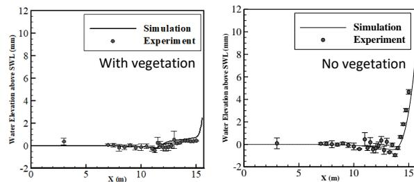
Figure 2. Comparisons of mean water surface elevations with and without vegetation
