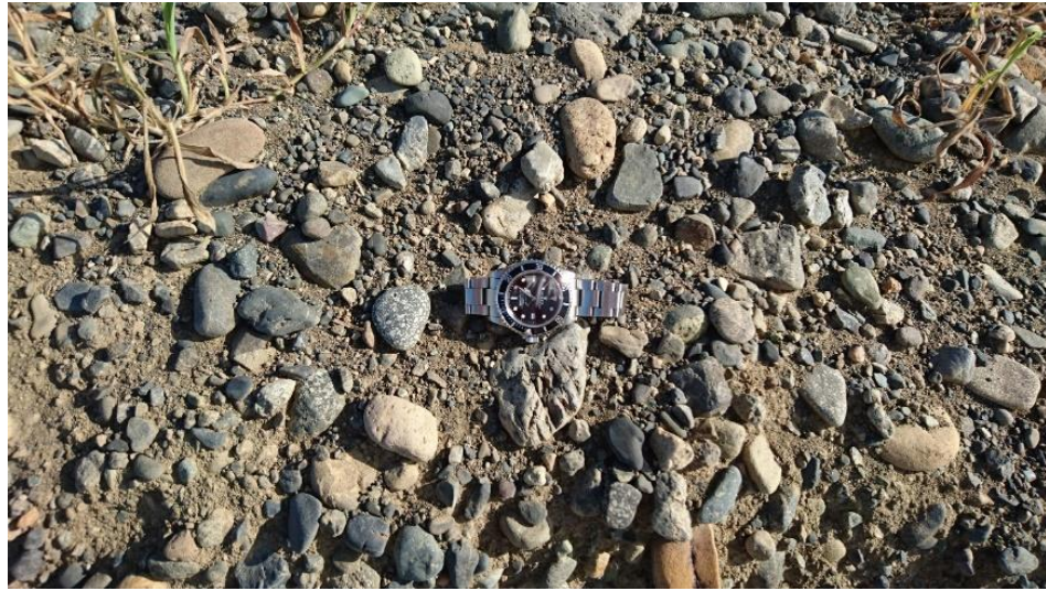
Figure 4. Material composed of gravel and sand for beach nourishment (August 16, 2016).
