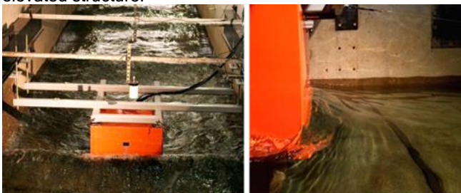
Figure 1 - Nonbreaking wave impacting test specimen: front (left panel) and side views (right panel).
