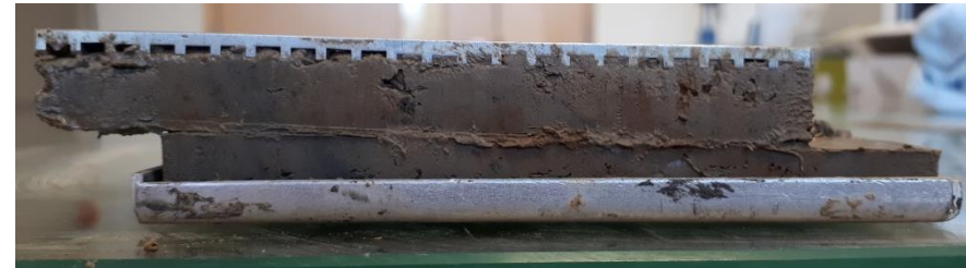
Shear plane created by shear box test. Taken: Dec 2017.
