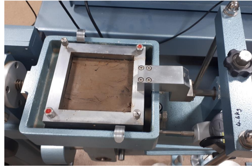
Sample preparation for shear box test. Taken: Feb 2018.
