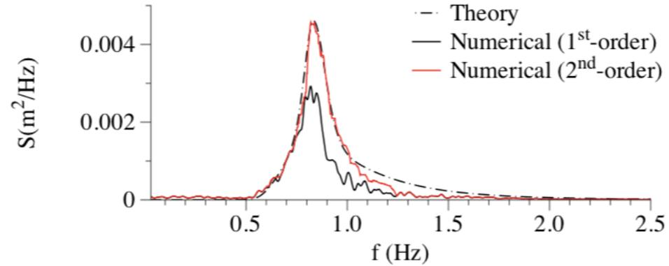
(b) Wave Gauge at  $x = 11\text{m}$
