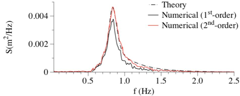
(a) Wave Gauge at  $x = 2\text{m}$
