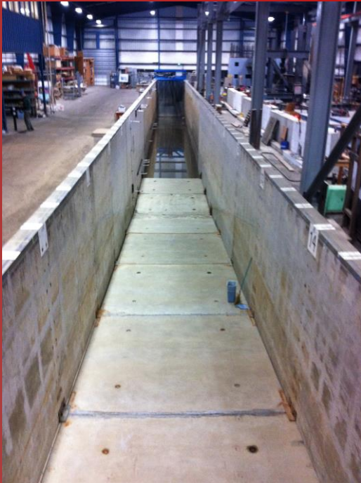
Large Wave Flume (104 m x 4 m x 5 m) Oregon State University
