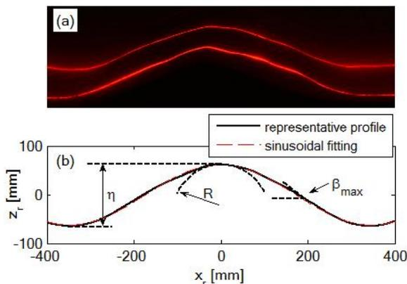
Figure 1 (a) laser image of a 2D equilibrium ripple
