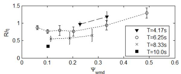
Figure 2 variation of  $R/\eta$  with Shields parameter
