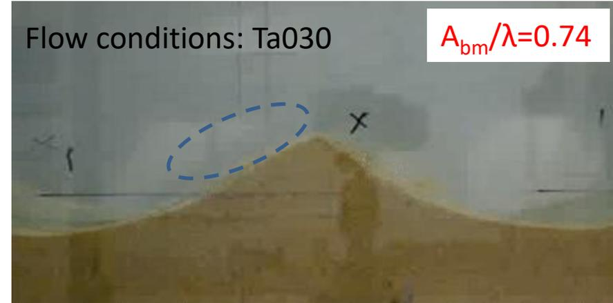
Flow conditions: Ta030  $\psi_{wmd} = 0.062$   $Re_w = 8.66 \times 10^4$   $A_{bm} = 30 \text{ cm}$   $\lambda = 39.8 \text{ cm}$
