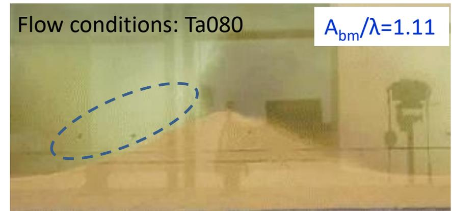
Flow conditions: Ta080  $\psi_{wmd} = 0.333$   $Re_w = 6.16 \times 10^5$   $A_{bm} = 80 \text{ cm}$   $\lambda = 71 \text{ cm}$
