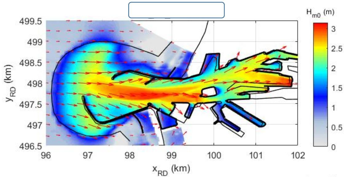
Wave growth  $E_G$  on top of penetrated wave field in PHAROS domain
