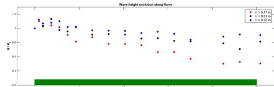
Figure 2 - Wave height evolution for regular waves ( $H = 0.06$  m,  $T = 1.2$  s) over  $h = 0.17, 0.33$  and  $0.50$  m.
