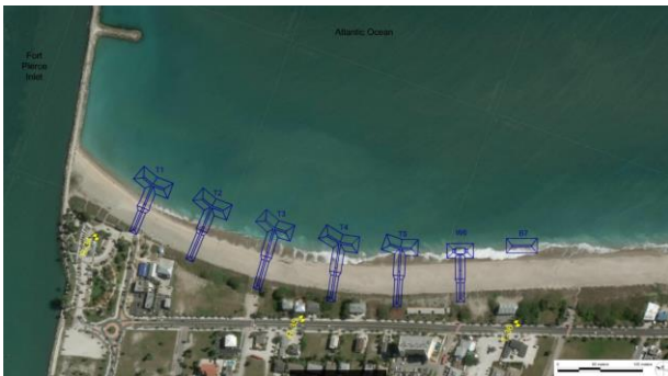
Figure 2 - T-head groins, T-head weir, and breakwater structures combined with beach nourishment for shoreline stabilization
