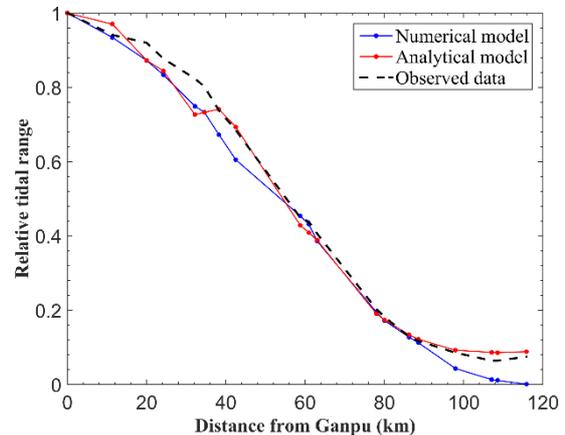
Figure 4 Comparison of the analytical and numerical results of the second bed friction method against the observations
