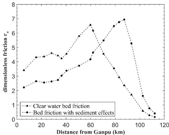
Figure 3 Dimensionless bed friction for clear water and sediment effect approaches respectively
