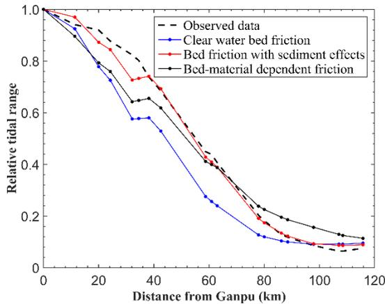
Figure 2 Analytical model results of different bed friction methods against the observations
