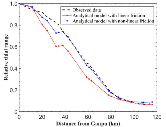
Figure 1 Comparison of linear and non-linear friction model results with observations
