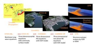
Figure-1 Overview of calculation system of Multiscale Multiphysics Integrated Simulator, STOC-CADMAS-STR
