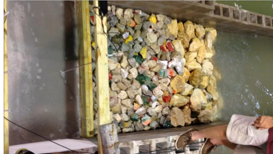
NOTE LACK OF PONDING CONTROLLED BY CUTOFF WALL AND DRAINAGE MANAGEMENT
