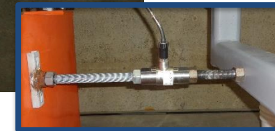
In-line load cell (for longitudinal forces)
