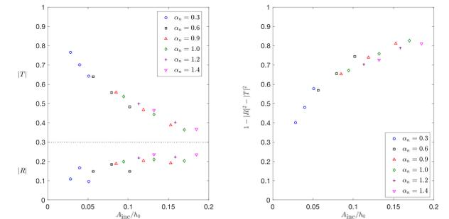
Figure 3 - Comparisons of reflection  $|R|$  and transmission coefficients  $|T|$ .  $1 - |R|^2 - |T|^2$  shows the percentage of energy dissipation by the forest.
