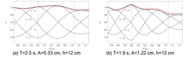
Figure 1 - Comparison of wave amplitude variation. Dashed lines show snapshots of dimensionless free surface while solid lines denote the upper wave envelopes. Diamonds present the linear model solutions.
