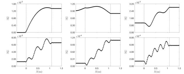
Figure 2 - Wave amplitude variation for each mode ( $T=2.5$  s,  $A=0.33$  cm,  $h=12$  cm)
