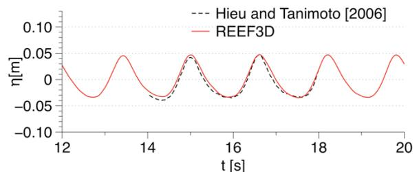
Figure 2 - Free surface elevation at WG1, upstream of the porous submerged breakwater showing the incident waves
