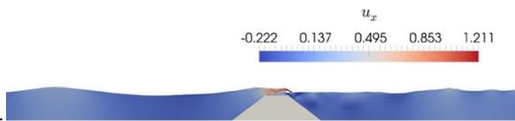
Figure 6 - Breaking wave on the crest of the submerged porous breakwater
