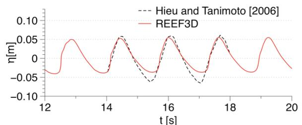
Figure 3 - Free surface elevation at WG3 on the crest of the seaward slope of the submerged breakwater
