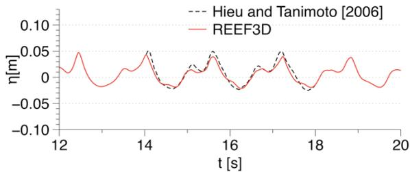
Figure 5 - Free surface elevation at WG6 at about L/2 from the toe of the leeward slope of the submerged breakwater
