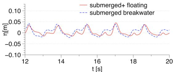
Figure 7 - Free surface elevation at WG6 at about L/2 from the toe of the leeward slope of the submerged breakwater, with and without the floating breakwater on the lee side.
