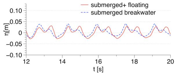
Figure 8 - Free surface elevation at WG7, a location just in front of the floating breakwater, with and without the floating breakwater on the lee side.
