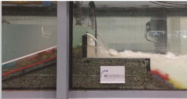
Figure 1. Overtopping over RMB with crown wall.
