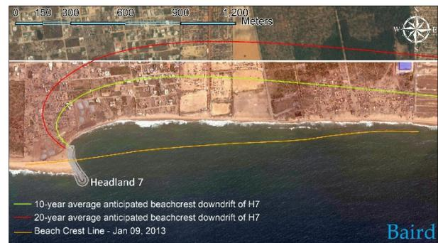
Figure 6 - Shoreline erosion conditions downdrift of Headland 7 in April 2018 vs. 10-year and 20-year predictions.
