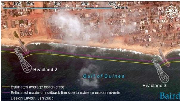
Figure 3 - Design vs. constructed Headlands 2 and 3 locations. The shoreline eroded approximately 100 m between completion of design and start of construction
