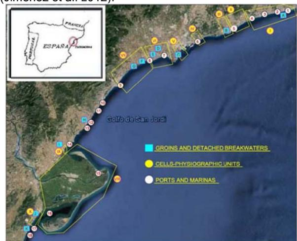
Figure 1 - Location of cells, ports and marinas, and protection beach works
