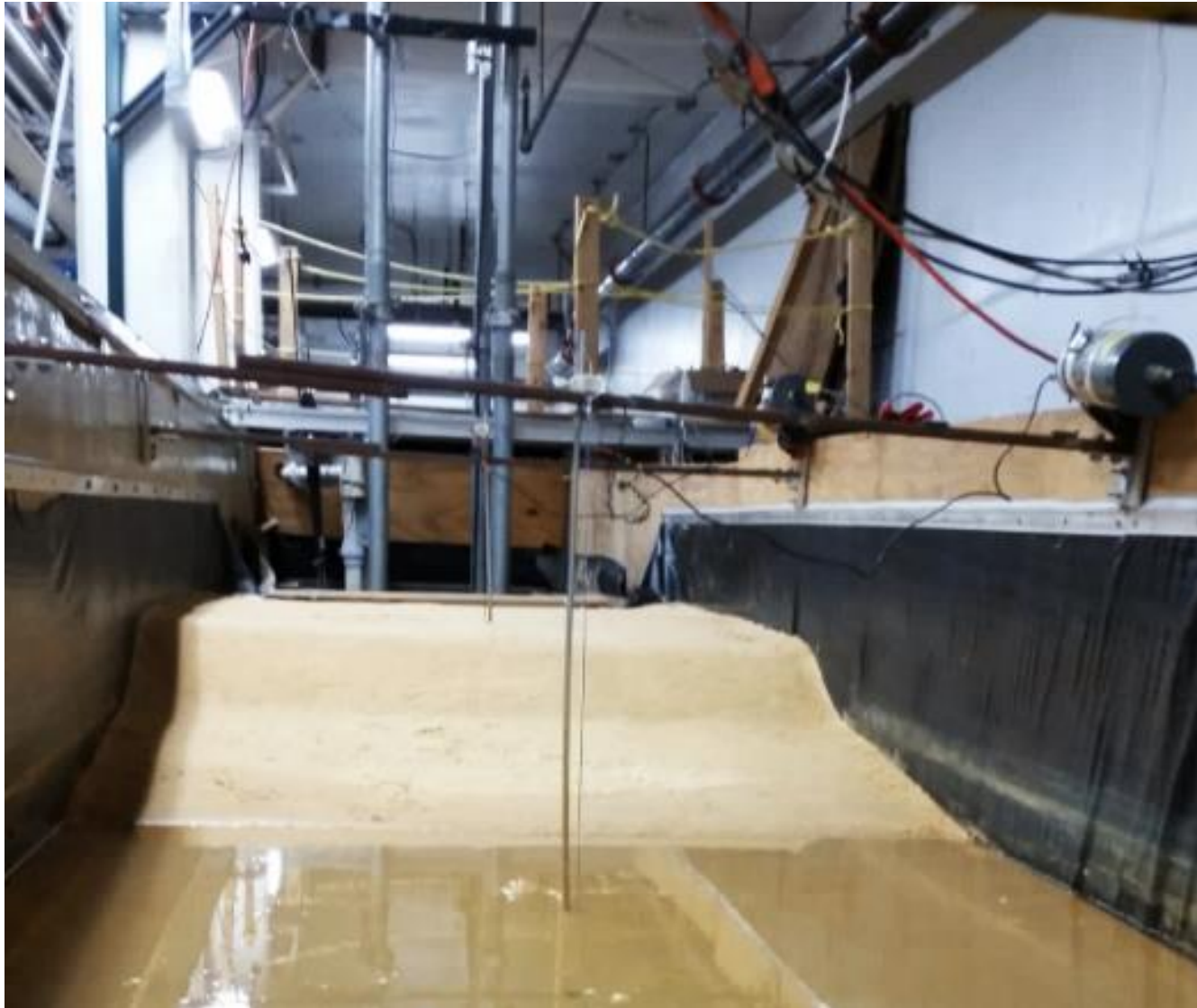
Berm in no protection test N
