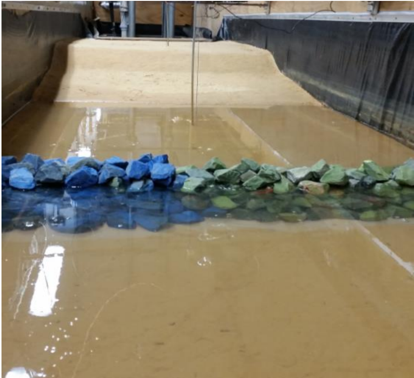
Berm protected by sill in test S
