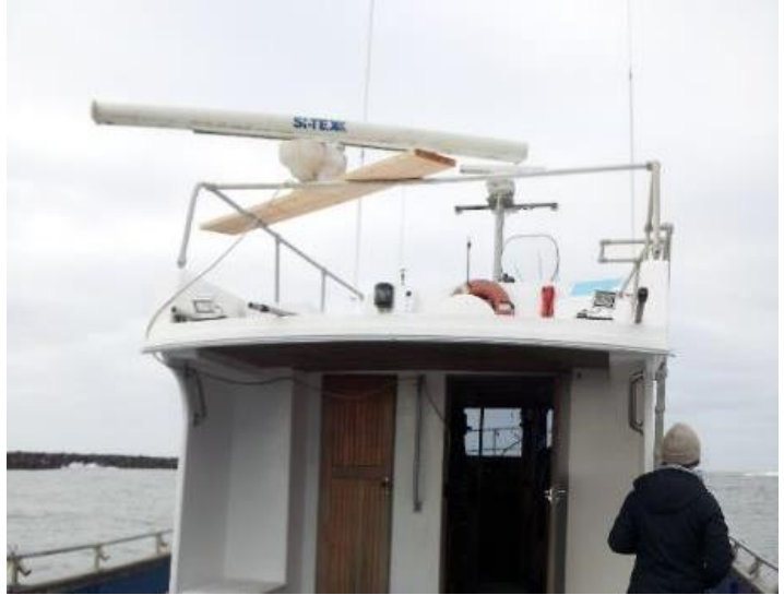
Vessel-based Radar Height < 10 m
