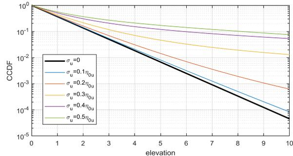
Figure 2 - Shift in mean flood hazard elevation due to uncertainty;  $\sigma$  denotes standard deviation of uncertainty (e.g. model error), lines are (complementary) cumulative distribution functions (i.e. flood hazard curves) with uncertainties proportional to the surge elevation  $\eta$
