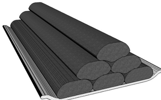
Figure 8. Geotextile Tube as a core of Breakwater
