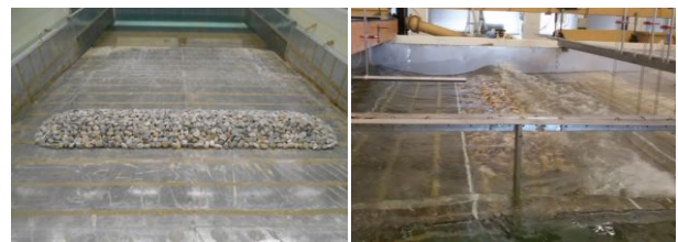
Figure 1 - Physical model of a low crested rubble mound breakwater with a zero free board.
