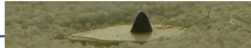
Ferrofluid located on a small cylinder ( $\phi=1,4$  cm) , to control its position on the sandy bottom
