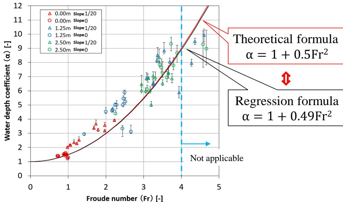
Relations between the water depth coefficient and the Froude number when the specific energy becomes the maximum
