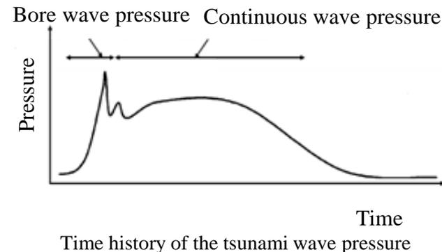
It is necessary to evaluate the tsunami design load appropriately with consideration of characteristics of such tsunami wave pressures.
